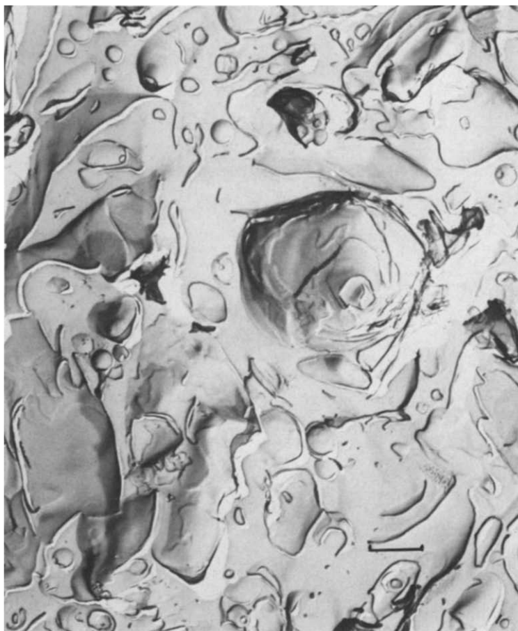
Fig. 5. Freeze-etch electrograph of the 2.5% w/w cetostearyl alcohol ternary gel ( T_4 ). Bar = 2 \mu m.
