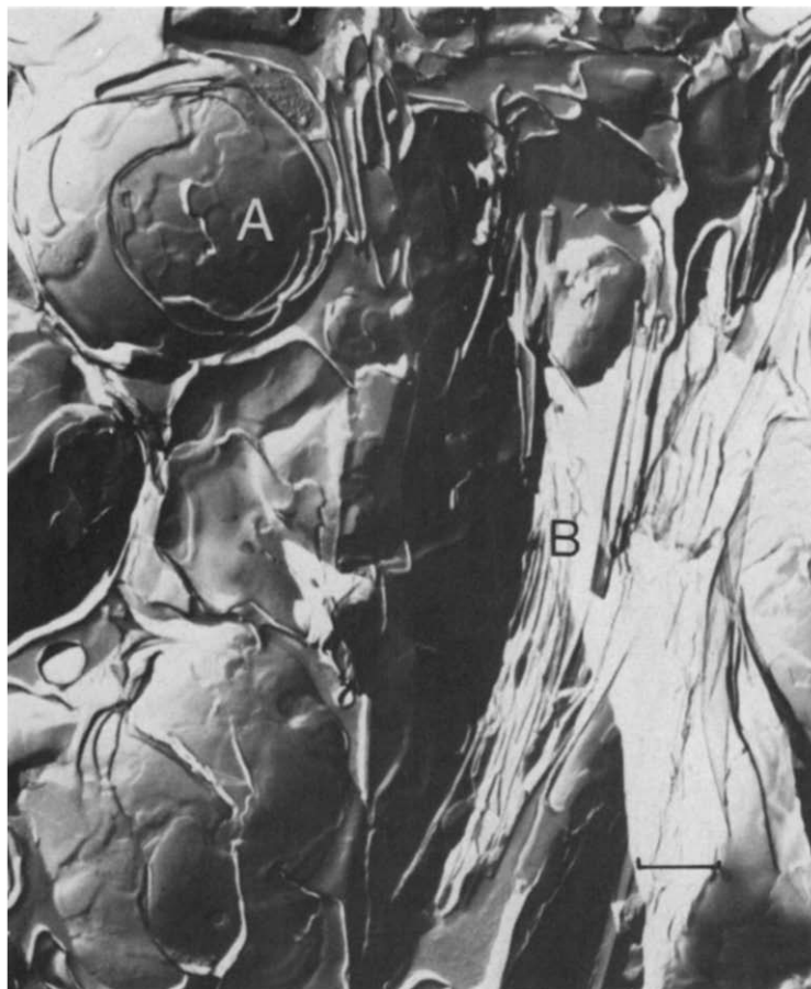
Fig. 8. Freeze-etch electrograph of an emulsion ( E_3 ) containing 20% oil. Note the oil droplets (Feature A) and the lamellar liquid crystalline network (Feature B). Bar = 2 \mu\text{m} .
