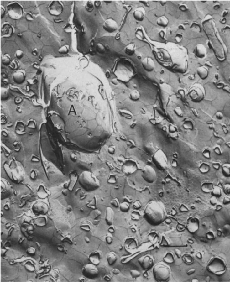
Fig. 4. Freeze-etch electrograph of the 1% w/w cetostearyl alcohol ternary gel ( T_3 ). Note the marked vesicular structure and features such as A which are believed to be due to excess cetostearyl alcohol. Bar = 2 \mu\text{m} .
